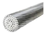
Designed to meet any international standards, these bare overhead conductors are used in primary and secondary distribution. All Aluminium Alloy Conductors (AAAC): These are made out of high strength Aluminium-Magnesium-Silicon alloy. As compared to conventional ACSR, AAAC are of
